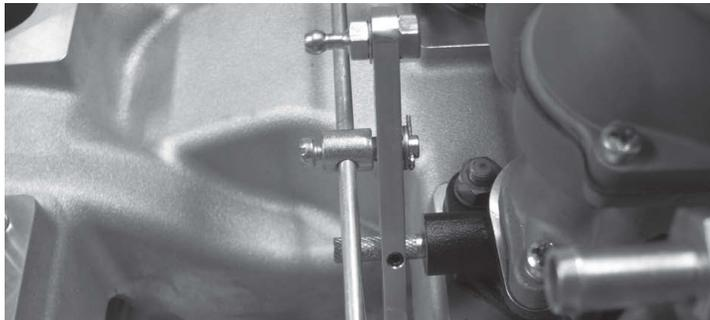
9. Install the three remaining carburetors on the driver side bank.
