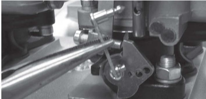
**NOTE:** All adjustments made to the carburetor arms should be conducted with all carbs at the wide open throttle position to ensure synchronized operation of such.
