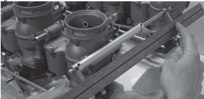
19. Attach the second spring-loaded throttle rod to the ball end stud on the driver side center carb throttle arm. Slide a swivel stud onto the driver side throttle rod and insert the swivel stud in the hole on the driver side control arm. Retain it with a washer and cotter pin, then tighten the swivel stud set screw.
