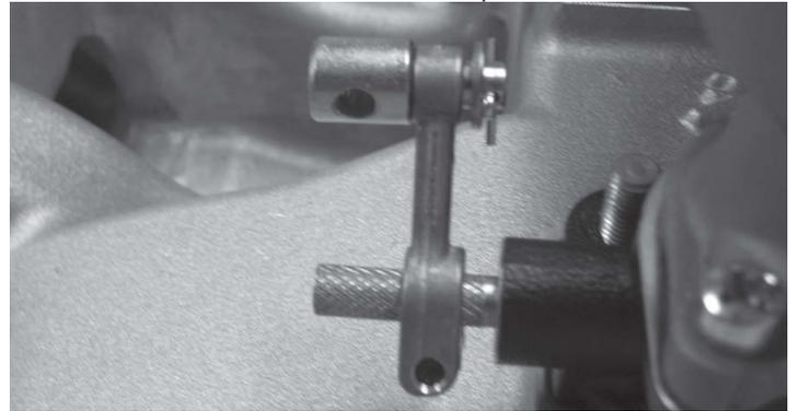
5. Verify that all three throttle arms are parallel by laying a straight edge across the swivel studs and measuring the distance between the straight edge and the bench at both the front and rear of manifold. It is recommended to start by aligning the front and rear arms without the center swivel stud in place. Once the two end arms have been determined to be parallel, add the center carb swivel stud and rotate the arm until the center swivel stud contacts the straight edge.
