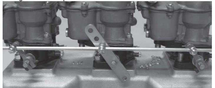
8. Install the ball end stud in the uppermost hole on the center carburetor throttle arm with the ball end extending away from the carburetor. Secure it with a star washer and nut.
