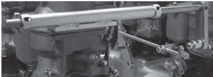
14. Connect the spring-loaded end of the throttle rod to the ball end stud on the passenger side center carburetor throttle arm, then push the center carburetor to wide open throttle and slide the opposite end of the throttle rod into the swivel stud on the passenger side control arm. With the passenger side carburetors still at wide open throttle, tighten the swivel stud set screw so that the control arm is pointing forward and down at a roughly 45° angle.
