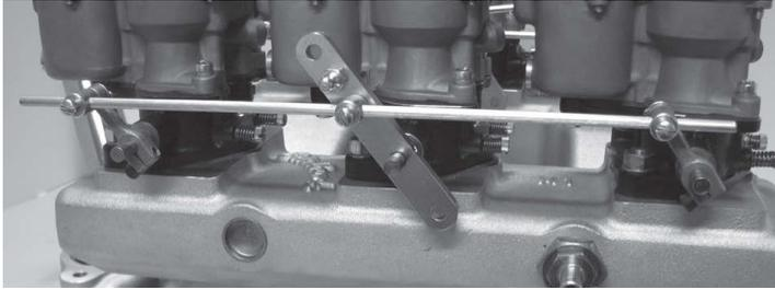
18. Likewise, install the driver side carburetor bank control arm. Loosen the collar set screws and readjust the position of the shaft, if necessary. Gently snug the set screws on the control arm and fully tighten the collars. Both bank control arms must be oriented at the same angle. To achieve this, use a straight edge across the back of arms and rotate one until the straight edge lays flat across them. Once properly aligned, fully tighten the set screws.
