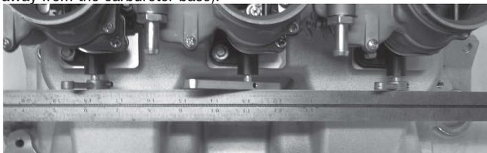
4. Once the correct depth and roughly equal angles have been achieved, install a swivel stud in each of the throttle arms with the threaded end pointed away from carburetors. The swivel stud on the center carb will go in the lowest of the three holes. Slide a washer over the back of the swivel studs and secure them with a cotter pin.
