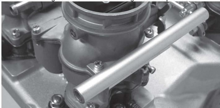
11. Slide the shaft into its housing. Slide a collar onto each end of the shaft so that they butt up against the housing.
