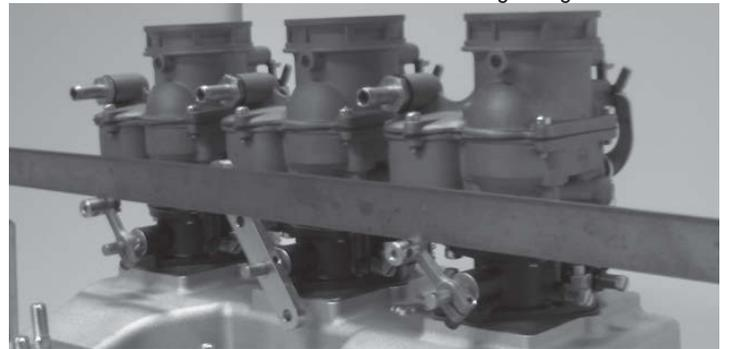
6. Once all three arms have been verified as parallel, tighten the set screws fully to secure the arms to their respective shafts. Twist each arm to ensure that the arms will not slip on the shafts.
