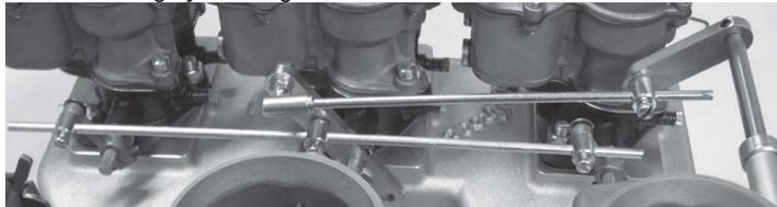
15. Mock up the distributor and spark plug wires in the manifold to ensure that the passenger side control arm and swivel stud can be operated throughout their full range of motion. (If the end of the throttle rod hits, it can be clipped off later.) Next, attempt to push the linkage past full throttle to be sure that bank control arms will not go over center and become inverted, and thus locked wide open.
