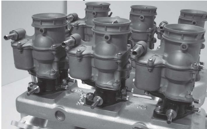
10. Remove the two air horn mounting screws at the back of the rear carburetor on the driver side and install the shaft housing. Replace the air horn mounting screws with the two longer screws provided.
