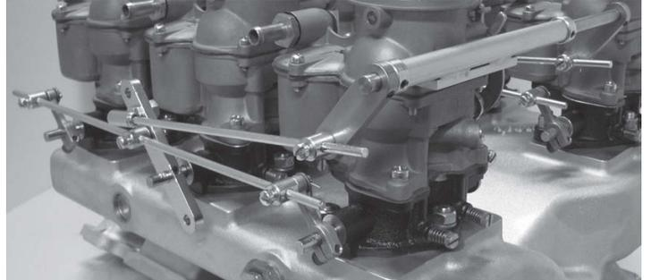
21. Cut rod ends to length, then mock up the distributor and plug wires once again to verify that nothing interferes with the linkage throughout its full range of motion.
