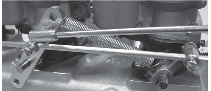
25. Install the X1 manifold according to the instructions supplied, then attach the vehicle throttle rod or cable to the ball end stud on the throttle linkage control arm. With the fuel system disconnected to prevent flooding, have an assistant depress the accelerator pedal to full throttle and allow it to return to idle several times to ensure that there is no interference or binding with the throttle linkage.
