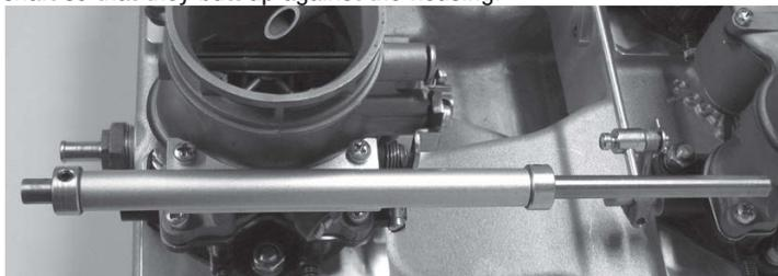
12. Place a swivel stud in one of the carb bank control arms and secure the stud with a washer and cotter pin.
