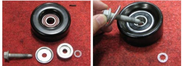
76. Apply Loctite to the threads on both idler pulley bolts. Then use a 15mm socket to install the 76mm idler pulley with the factory hardware to the left idler pulley location. Install the additional idler pulley to the right idler pulley location with the M8 x 20mm bolt and M8 washer from Bag #1. Verify that both pulleys spin freely.
