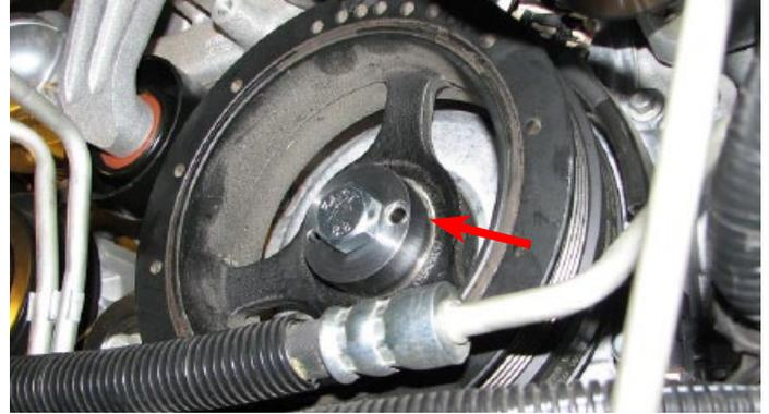
17. Measure 1.7" from the tip of the 15/64" drill bit supplied in Bag #4 and mark the position with a piece of masking tape. Drill into the crank through the hole in the guide that has a bushing in it, stop when the tape mark reaches the drill guide.
