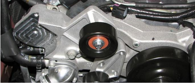
71. Apply blue Loctite to the threads of the M10 x 75mm Hex flange bolt supplied in Bag #1. Use a 15mm socket to install the supplied tensioner onto the tensioner bracket.
