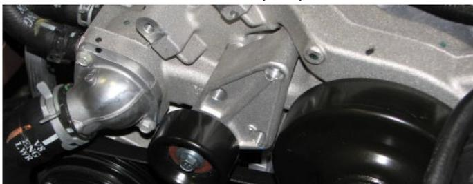
66. Use a 15mm socket to remove the nut retaining the ground strap on the passenger side cylinder head then use a 15mm deep socket to remove the ground strap stud.
