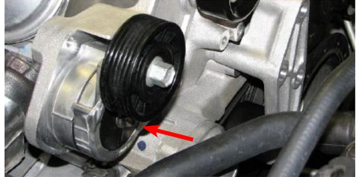
60. Route the serpentine belt (*not included*) according to the diagram below. Note that you must slide the belt around the bottom of the bracket to get the belt on the lower passenger side idler pulley.
