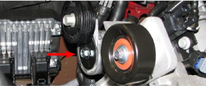
72. Use a 12mm socket and an M8 x 20mm bolt supplied in Bag #1 to secure the ground strap to the back side of the tensioner bracket.
