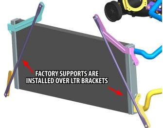
45. Using the factory bolts, reinstall the factory core support braces over the LTR brackets. Be sure to add the M12 spacers between the upper LTR brackets and core support brace.
