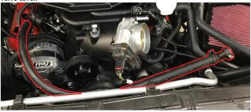
36. Place hose clamps inboard of all hose ends. Install hoses onto the LTR as pictured. Coolant ports should face the driver side with ports positioned towards the rear. **NOTE:** Position hose clamp tabs so they face the rear of the
