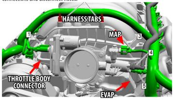
11. Remove (2) hose clamps and (1) PCV hose from the intake tube and remove.
