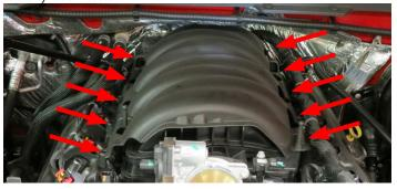
15. Pull the intake out to access the (3) rear harness retainers and detach harness from rear of intake.
