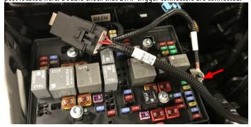
54. Fasten the ground lead underneath the ground post located on the passenger side fender near the hood shock. Secure wiring away from pulleys.
