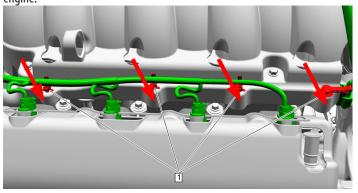
14. Using a 10mm socket, remove ten (10) bolts securing the intake manifold to the cylinder heads.
