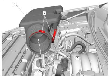
12. Disconnect the (3) harness retainers from the driver's side of the engine.
