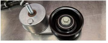
27. Using a 15mm socket, install the tensioner using the supplied 75mm bolt and a M10 washer.
