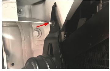
8. Remove (2) cross support bars using a 15mm socket. Set aside. These will be reused.
