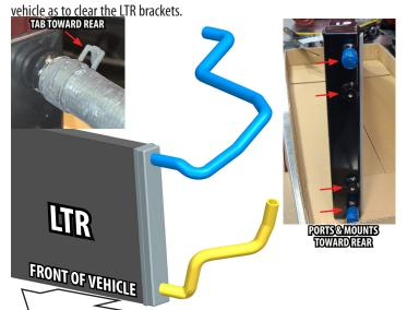
37. Feed LTR hoses through the gap in the core support located on the driver's side of the radiator. **NOTE:** Protect the LTR from damage from the lower center shutter support
