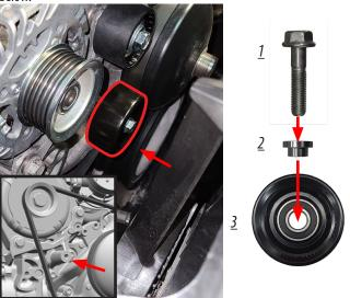
29. Place the M10 x 110mm bolt, 22mm 0D washer into the smooth idler provided in this kit. Place the M10 aluminum boss onto the opposite side as pictured below.
