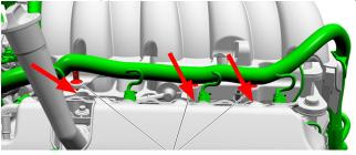
13. Disconnect the (4) harness retainers from the passenger's side of the engine.
