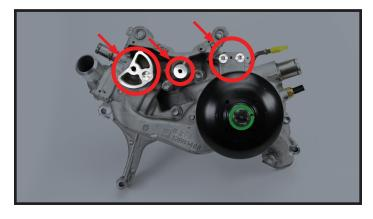
If your truck does not have the pump with the machined surface and threaded holes like the one on the right, you will need to replace the water pump before proceeding with the supercharger installation.
