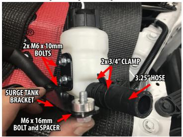
42. Install the surge tank assembly to the rearward port on the supercharger. Bolt the bracket underneath the supercharger lid.
