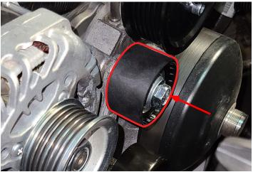
31. Using a 15mm socket, remove the vestigial grooved idler on the driver's side of the engine. Or you may leave it installed. In either case it will no longer be used.
