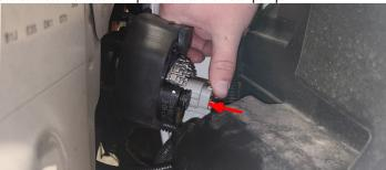
53. Connect the Water Pump Harness 12V positive lead to the 12V positive post located here. Double check that EVAP trigger connectors are connected.
