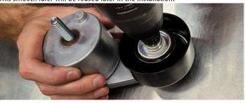
26. Using the same bolt removed in the previous step, apply Red loctite to the bolt, and install the supplied grooved idler pulley to the tensioner using the supplied M8 washer.
