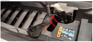
3. Remove 10 clips holding the upper radiator cowl in place. Remove cowl.
