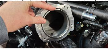
24. Reinstall the throttle body using the provided (4) M6 x 40mm bolts. Check to make sure the throttle body is in the correct orientation.
