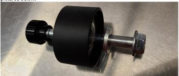
30. Swing alternator back into position. Install idler and 110mm bolt assembly into the alternator mount using Blue Loctite. This bolt will replace the one that was removed earlier in this install.
