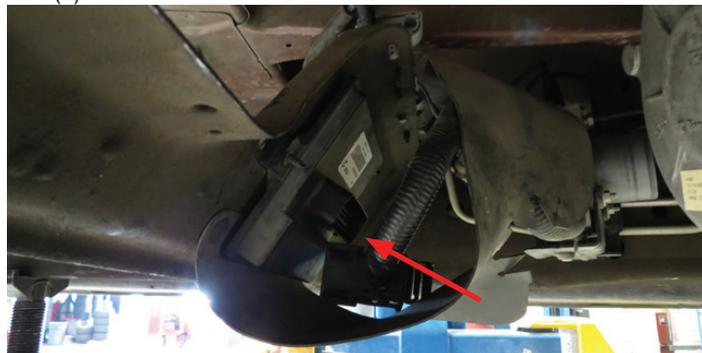
25. Unplug the chassis harness from the fuel pressure control module.
