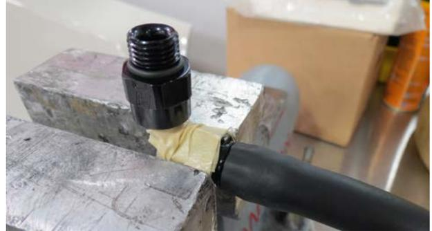
5. If the hose is not able to be pressed onto the fitting, repeat step #3 and try again. If the hose is only able to be partially installed on the fitting, remove the hose by cutting it with a razor blade parallel to the fitting. Trim the hose end to remove the cut left by the razor blade and go back to step #3.
