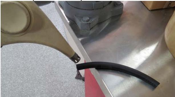
4. While the hose end is hot, push the hose onto the fitting using one, quick motion to fully seat the hose on the fitting so it reaches over both fitting barbs. If the hose is fully seated on the fitting, proceed to step #6.
