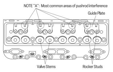
Figure 4 - Pushrod Guide Plate Clearance
