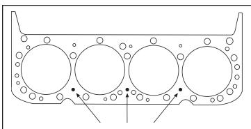
Drill three .125" holes in each head using 400 c.i.d. head gasket as a guide. **DRILL ONLY THE THREE LOWER STEAM HOLES** (closest to the spark plugs) as indicated. Drill straight into the head (90° from the deck) until the drill breaks through into the water jacket (about 9/16").
